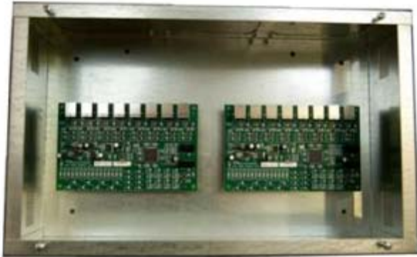
Figure 41: System Network Hub with Redundant PWA's
