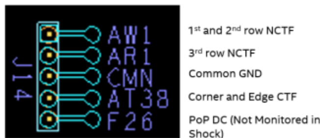
Figure 10. Daisy chain net designators for Shock and Temp cycle coverage. NCTF = Non critical to function; GND = Ground; CTF = Critical to function
