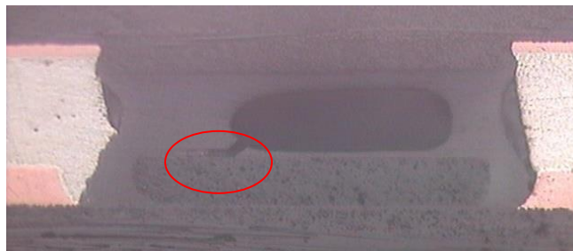
Figure 29. Evidence of Dis3 material crack initiation site in the SJEM cured Resin
