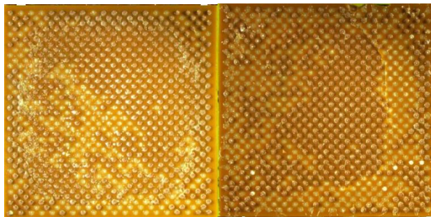
Figure 17. SJEM Dispensing Material Coverage (Left: Dis1; Right: Dis2)
