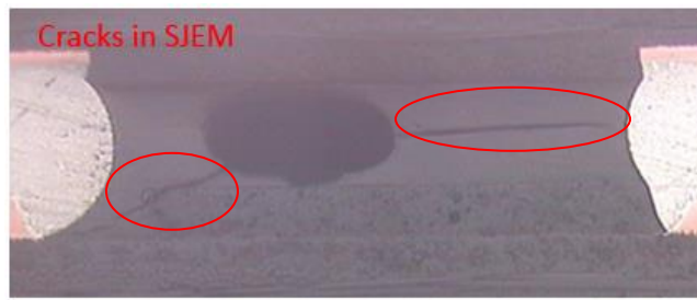
Figure 28. Evidence of Dis2 material crack initiation site in the SJEM cured Resin
