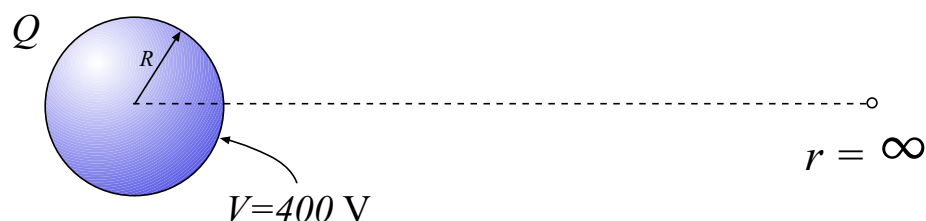
Figure 4.4: Conducting charged sphere, has potential of 400 V (with V = 0 at r = \infty ), from Example 8.
